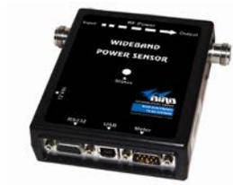
The best solution for measuring TDMA signals is to measure burst average power with the duty cycle. Burst average power will give you the average power of all the active slots and duty cycle will tell you how many slots are active. This measurement would be able to flag any kind of decay in pulse power, inactive slots, and misalignment of signals that might occur. This measurement can also be made on a "live" signal without affecting the accuracy.
